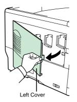
2 While holding the waste toner box, press the lock lever and then gently remove the waste toner box.
